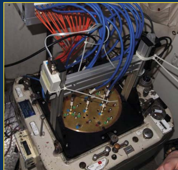
The SAMI plug plate assembly unit mounted onto the Prime Focus Camera. The white "splice box" connects the blue hexabundles and orange sky fibres from the brass plug-plate to the fibre bundle.
