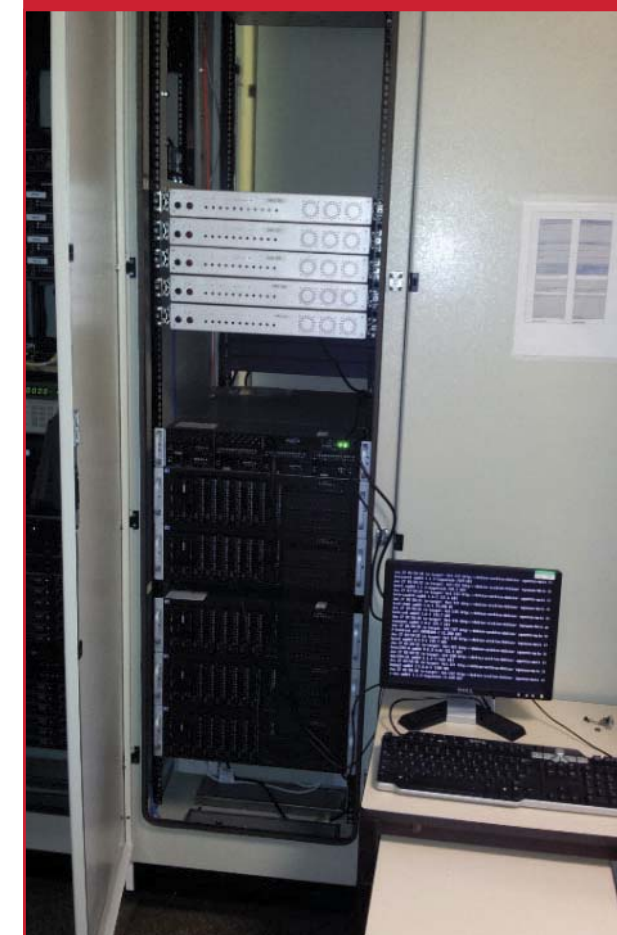
The server for the new HI and Pulsar (HIPSR) machine. The silver boxes at the top of the rack are Reconfigurable Open Architecture Computer Hardware (ROACH) boxes, developed by the Collaboration for Astronomy Signal Processing and Electronics Research (CASPER) group at UC Berkeley. Some of the additional data processing machines can be seen in the bottom of the rack. Jonathan Kocz
