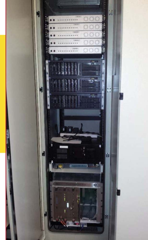
The server for the new HI and Pulsar (HIPSR) machine. The silver boxes at the top of the rack are Reconfigurable Open Architecture Computer Hardware (ROACH) boxes, developed by the Collaboration for Astronomy Signal Processing and Electronics Research (CASPER) group at UC Berkeley. Some of the additional data processing machines can be seen in the bottom of the rack. Jonathan Kocz
