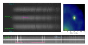
WiFeS "slices" a 25" x 38" field of view into 25 1"-wide "slitlets" by means of a fanned segmented mirror. Light in each slitlet is dispersed in the same manner as a longslit spectrograph, but ultimately yields a data volume 25 times that of a standard longslit spectrograph. Calibrating this volume of data is a challenging task, but one well suited to recursive software techniques such as PyWiFeS that accomplishes endto-end processing of WiFeS data with minimal user interaction
