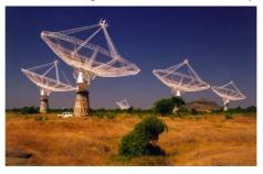
that is much more prone to radio frequency interference (RFI) than the SKA sites. The team exploited the GMRT's software backend option of recording raw voltage data (in two polarisations) from the individual array elements; they then dedispersed the data and searched for transient events by imaging known sources such as the Crab Pulsar.
