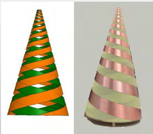
Dual-polarized conical spiral prototype
