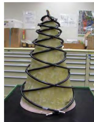
Dual-polarized wire conical spiral prototype
