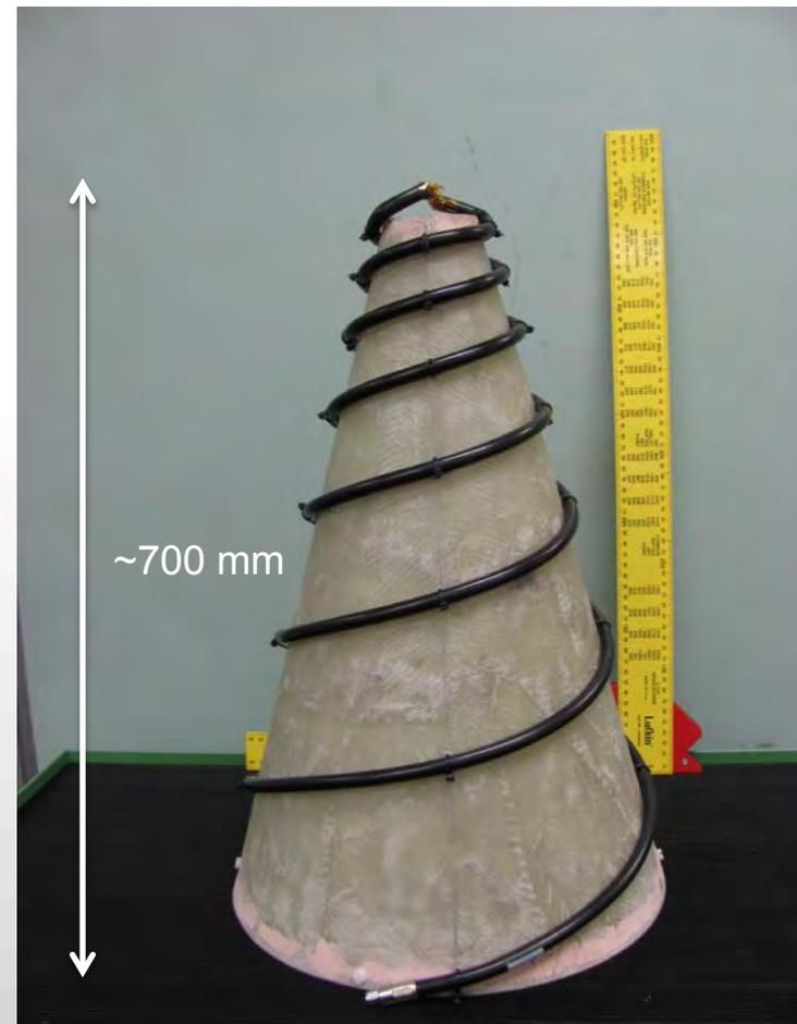
1/3 scale model of SKA-low conical wire spiral antenna
