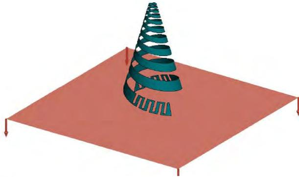
Meander conical spiral antenna
