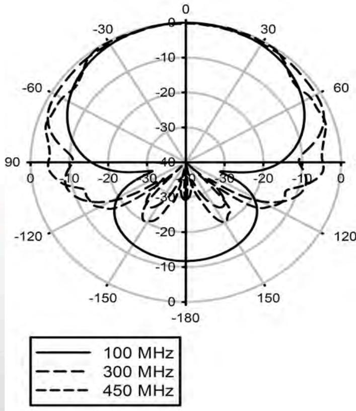
Radiation pattern of wire conical log spiral
